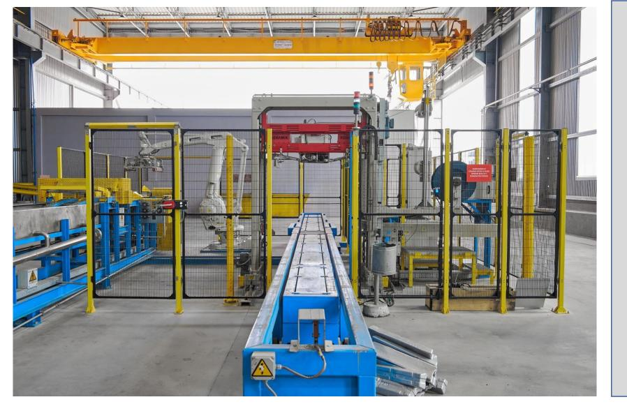
Robot arm assisted Automatic packing line 400-500 kg packing weight
